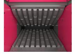
Deep 1.91m jaw chamber with single toggle design accommodates hard rock applications and large feed sizes. Also features closed side setting adjustment with hydraulic wedges.
