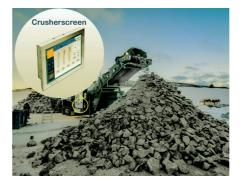
Standard telematic control system delivers machine data to a central dashboard for convenient monitoring of belt scales, automation system, generator/ engine, and alarm logs and diagnostics.
